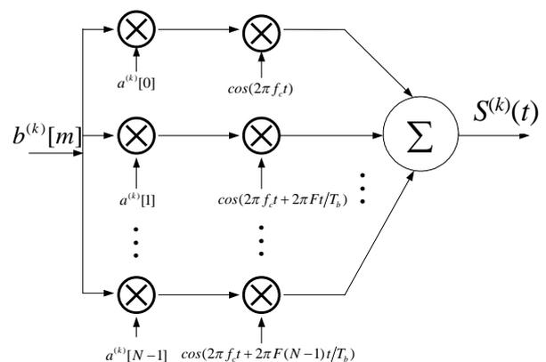
Fig. 1 The transmitter model of the MC-CDMA system
