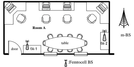
Fig. 1. Top view of the deployment of MIMO-FT in a living home
