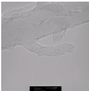
(b) Top-view TEM images of the CNTs grown on silicon nanowires
