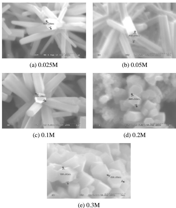
**Fig. 2.** The enlarged top-view SEM images of ZnO nanorods prepared by various concentrations of  $\text{Zn}(\text{NO}_3)_2 \cdot 6\text{H}_2\text{O} + \text{C}_6\text{H}_{12}\text{N}_4$ . The magnification factor is  $3 \times 10^4$ .
