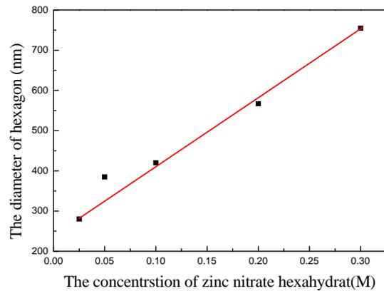
**Fig. 3.** Average diameter of ZnO nanorods prepared by various concentrations of  $\text{Zn}(\text{NO}_3)_2 \cdot 6\text{H}_2\text{O} + \text{C}_6\text{H}_{12}\text{N}_4$ .
