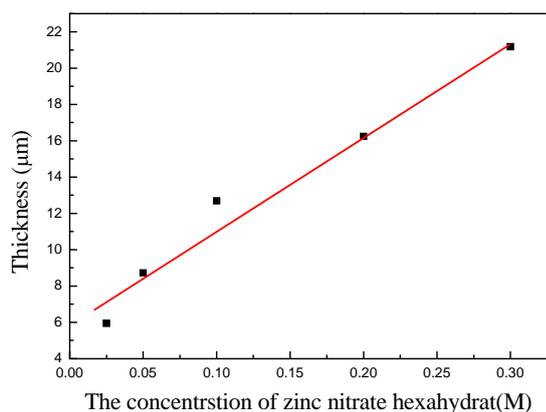
**Fig. 4.** Film thickness of ZnO nanorods prepared by various concentrations of  $\text{Zn}(\text{NO}_3)_2 \cdot 6\text{H}_2\text{O} + \text{C}_6\text{H}_{12}\text{N}_4$ .
