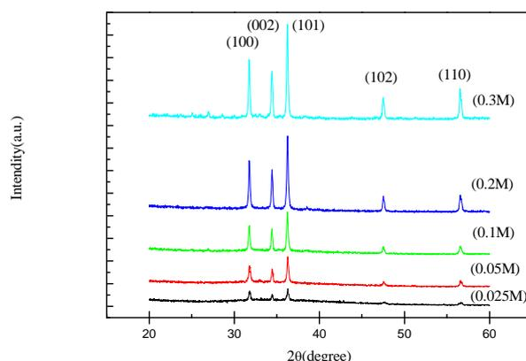
**Fig. 5.** XRD spectra for the ZnO nanorods prepared by various concentrations of  $\text{Zn}(\text{NO}_3)_2 \cdot 6\text{H}_2\text{O} + \text{C}_6\text{H}_{12}\text{N}_4$ .
