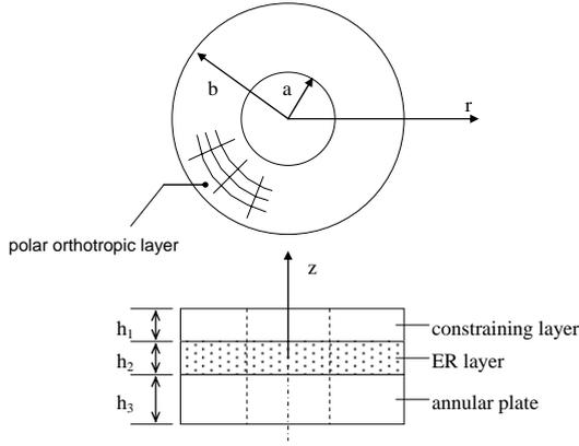
Fig. 1. Polar orthotropic sandwich annular plate system
