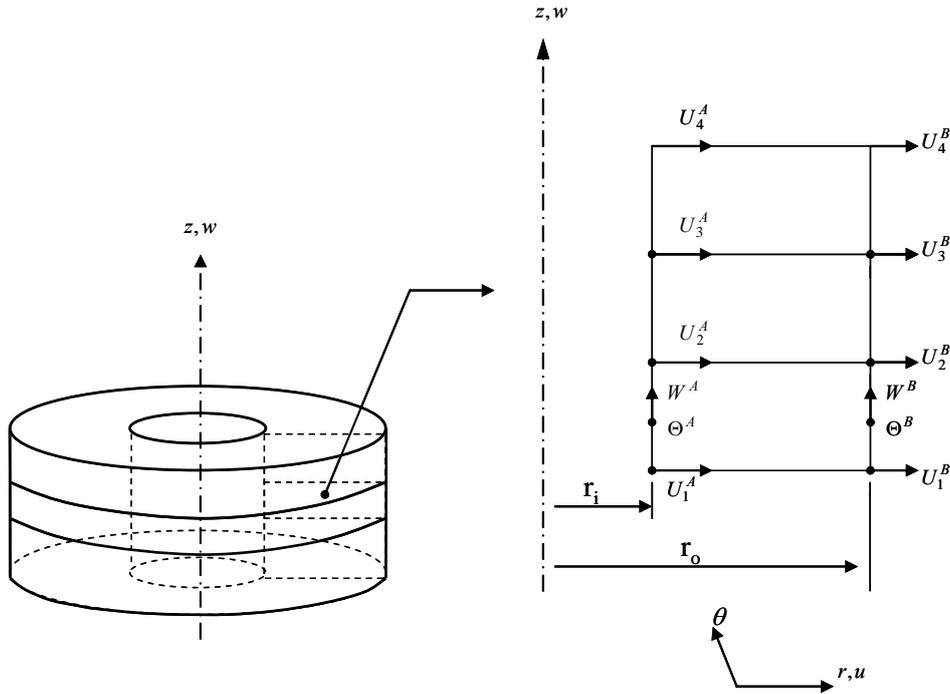
Fig. 2. Three-layer discrete layer annular finite element
