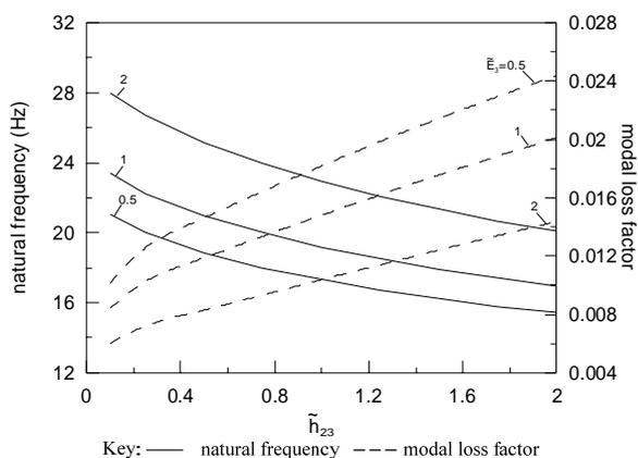
**Fig. 6. Effects of thickness of ER layer on the natural frequencies and the modal loss factors of the sandwich annular plate with various ratios  $\tilde{E}_3$**
